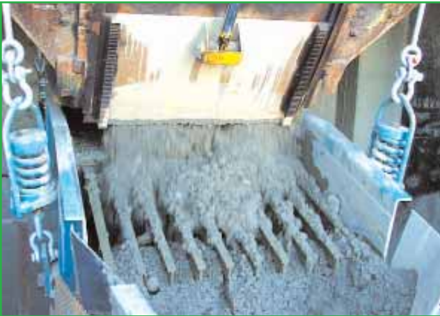
Jeffrey incorporated a scalper into the design of the feeder, a feature that is very beneficial to J.P. Sand.
